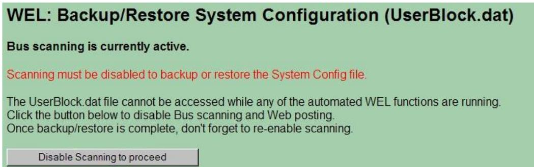
When saving or restoring the system configuration file, it's necessary to stop the WEL from performing active polling, which may attempt to read or write to the UserBlock.dat file. Simply click the **"Disable Scanning to Proceed"** button. At which point the following screen will be displayed:
