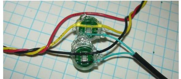
In some situations, it's just not convenient to have one single long bus for all the sensors. In these cases, one incoming cable might need to branch out to several sensors throughout the house (eg: at thermostat locations). Here, the various cables are connected in "parallel" to form a "Star" network. You MUST limit the number of stars in your system by deciding on a central hub location and only fanning out from there.
