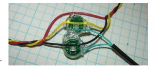
In some situations, it's just not convenient to have one single long bus for all the sensors. In these cases, one incoming cable might need to branch out to several sensors throughout the house (eg: at thermostat locations). Here, the various cables are connected in "parallel" to form a "Star" network. You MUST limit the number of stars in your system by deciding on a central hub location and only fanning out from there.
