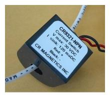
As its name implies, the CS is a switch that turns on when it senses current. This is a great way to detect when a device like a pump or heater element is on (it doesn't actually "measure" power usage).
