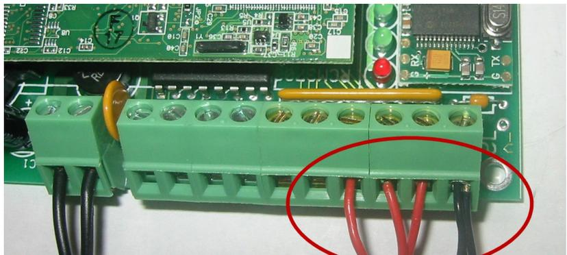
This photo shows 3 CS’s connected to the WEL as Run inputs 6,7 & 8.
