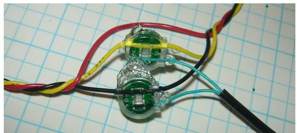
In some situations, it’s just not convenient to have one single long bus for all the sensors. In these cases, one incoming pair might need to branch out to several sensors throughout the house (eg: at thermostat locations). Here, the various pairs are connected in “parallel” to form a “Star” network. You should attempt to limit the number of stars in your system by deciding on a central hub location and only fanning out from there.
