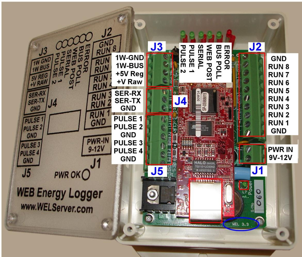
The previous picture shows the WEL 3.3 Unit in its preferred orientation. When the board is mounted to a wall in an enclosure, the six status LEDs should be located at the top of the board, and the Ethernet connector at the bottom. This orientation leaves the top surface of the enclosure free from
