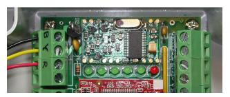
Here you see the Bus cable connected to the WEL using the standard color code.
