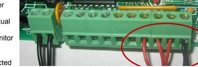
This photo shows 3 CS's connected to the WEL as Run inputs 6,7 & 8.
