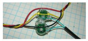
sensors throughout the house (eg: at thermostat locations). Here, the various pairs are connected in "parallel" to form a "Star" network. You MUST limit the number of stars in your system by deciding on a central hub location and only fanning out from there.
