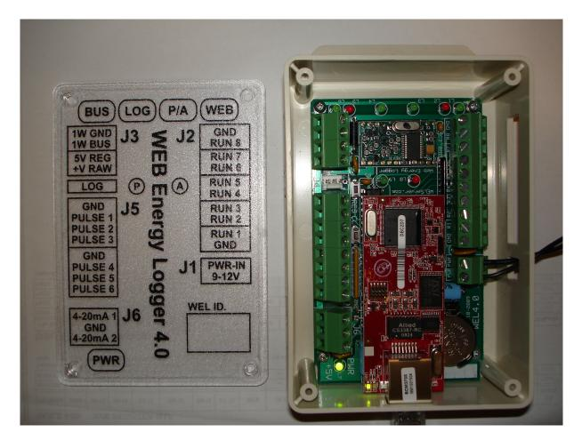
The picture shows a WEL 4.0 Unit in its preferred orientation. When the board is mounted to a wall in an enclosure, the four LED groups should be located at the top of the board, and the Ethernet connector at the bottom. This orientation leaves the top surface of the enclosure free from openings. The clear cover has a wiring legend, plus several status "bubbles" (oval areas that are illuminated from below). Green bubbles indicate activity; Red bubbles indicate some error condition.
