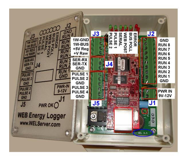
The previous picture shows the WEL 3.3 Unit in its preferred orientation. When the board is mounted to a wall in an enclosure, the six status LEDs should be located at the top of the board, and the Ethernet connector at the bottom. This orientation leaves the top surface of the enclosure free from holes. The version of the WEL is marked on the main circuit board, directly under the LAN connector. A WEL 3.3 board can also be identifiable by the stand-alone 4 terminal 1-Wire bus connector.
