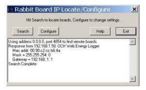
In the example, you can see that the program got a "Response from 192.168.1.50". This is the WEL's IP address. You'll also not that the Gateway address is 192.168.1.1, this is typical for many network routers (like Linksys). If need be, these addresses can be changed by clicking the "Configure" button and entering the desired addresses.
