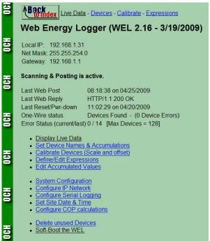
Below the network information is Web Posting and Bus Scanning status information. Scanning and Posting must be shown as "active" for the WEL to read the 1-wire bus and post data to the central server. The ONLY time scanning is disabled is when you (the user) disable it in order to delete some unwanted devices. If scanning has been disabled, there will be a red warning, and a button that can be used to re-enable it.
