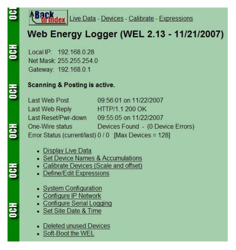
Below the network information is Web Posting and Bus Scanning status information. Scanning and Posting must be shown as "active" for the WEL to read the 1-wire bus and post data to the central server. The ONLY time scanning is disabled is when you (the user) disable it in order to delete some unwanted devices. If scanning has been disabled, there will be a red warning, and a button that can be used to re-enable it.
