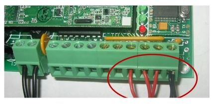
If it's not convenient to wire a CS directly to the WEL, or if you need to monitor more than 8 devices, I have developed a 1-wire interface for the Current Switch. This interface is wired to the CS, and provides the standard Black/Yellow wire pair that can then be connected anywhere on the 1-wire bus. This configuration can provide the ultimate in wiring convenience and flexibility. I call this my "1-wire Current Switch" (p/n WEL-CS)
